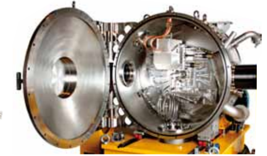
Fixed exit double channel DCM Monochromator (2.5÷100 keV) for ID06 Beamline European Synchrotron Radiation Facility - ESRF Grenoble (France)
