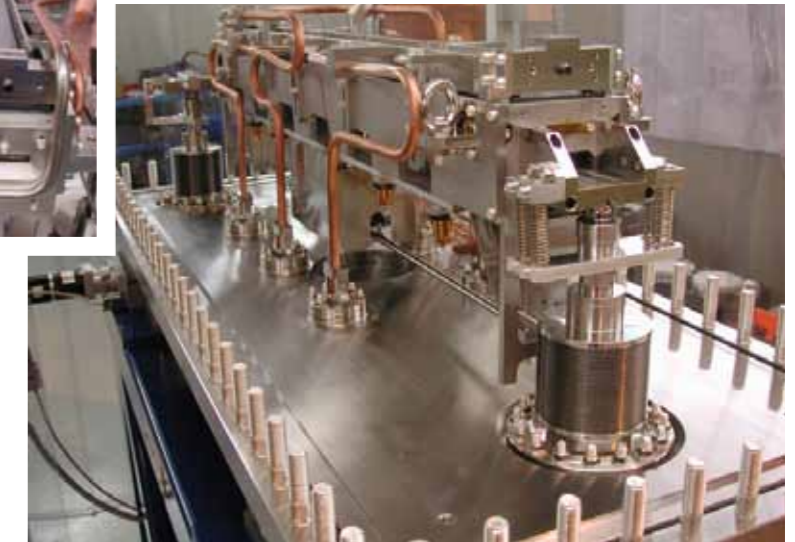
Mirror Chamber for Protein Crystallography Beamline (M1) X06DA Swiss Light Source - SLS Villigen (Switzerland)
